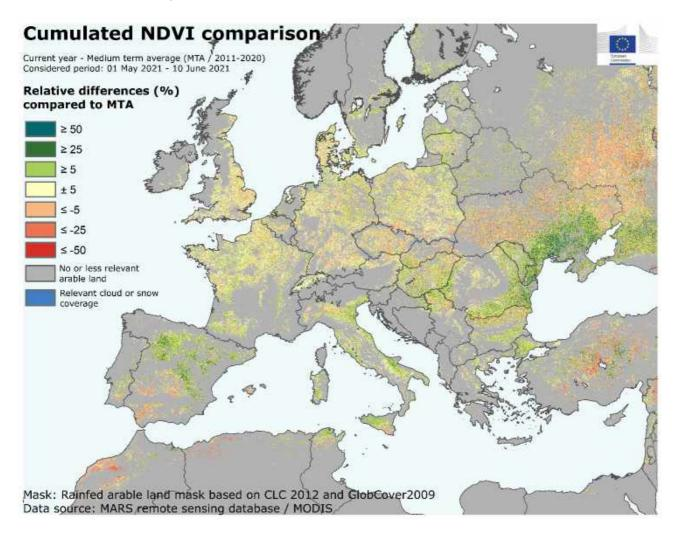
The map displays the differences between the Normalized Difference Vegetation Index (NDVI) cumulated from 1 May to 10 June 2021 and the medium-term average (MTA, 2011-2020) for the same period. Positive anomalies (in green) reflect above-average canopy density or early crop development while negative anomalies (in red) reflect below-average biomass accumulation or late crop development
